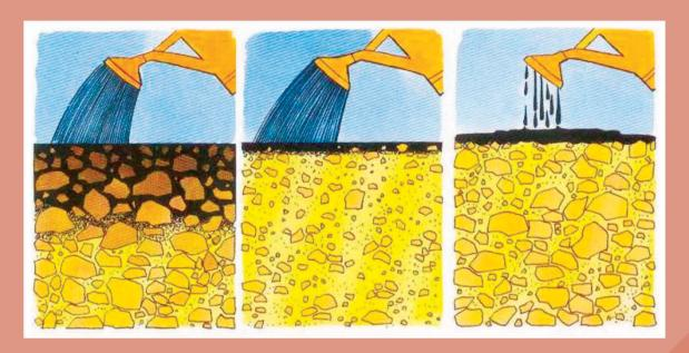
The emulsion must penetrate the first few millimeters of the layer very quickly
